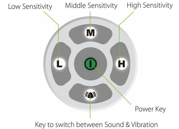
This detector has illuminated keys, which indicates its working state.
