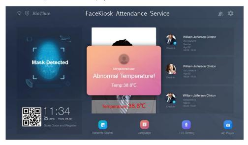
**Temperature Over the Range Access Denied:** When the detected temperature is higher than the high temperature alarm threshold, the device will deny user access.
