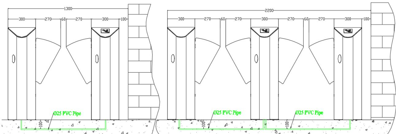
Figure 4-1A Single-Passage and Dual-Passage with FBL 4000
