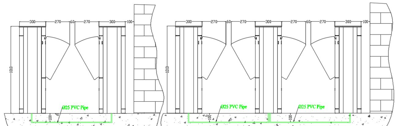
Figure 4-1B Single-Passage and Dual-Passage with FBL 5000
