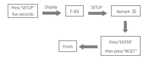
Remark ③: "xx" means working frequency ,press "SETUP" to select frequency, the scope for working frequency is 1-12 can be selected.
