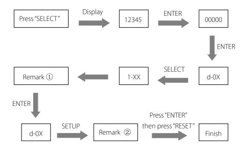
Remark ①: "1" means zone 1,press "SELECT" to select zone 2-7 to adjust corresponding zone sensitivity, especially zone 7 is whole sensitivity, "xx" is sensitivity level, press "SETUP" to adjust tens digit, press "ENTER" to adjust unit digit.(the bigger sensitivity levels the higher sensitivity)
