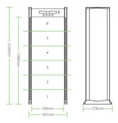
Input voltage: 100-240V, 50/60Hz Power: 12W
