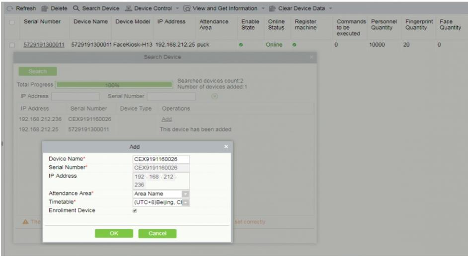
Set the IP address and the cloud service server address on the device before registering into the software.
