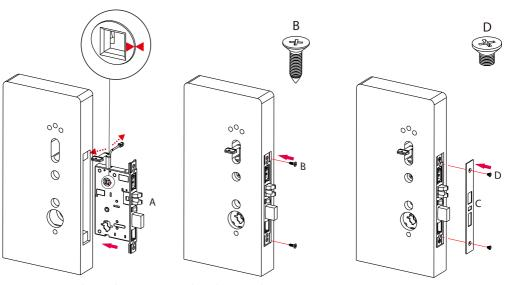
**Note:** Two Triangles on the mortise must be in horizontal alignment (as the above enlarged figure).
