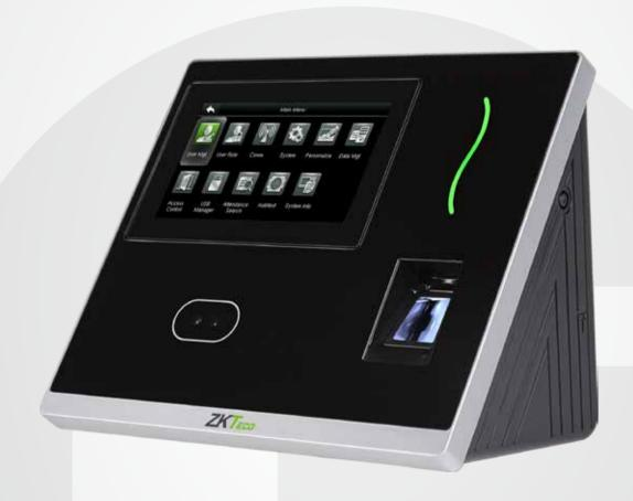
G3-H is a multi-biometric identification terminal which features ZKTeco's innovation Silk ID fingerprint sensor technology. With the world's cutting-edge 3D Neuron Fingerprint Algorithm, it precisely authenticates dry, wet, or rough fingerprints efficiently and accurately. Infrared technology enables the device to function automatically when fingerprints are detected. With the latest facial algorithm, it supports color photoes detection and prevents repeated face registration.
